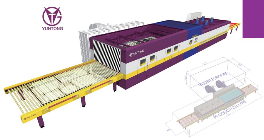
Pass-through quenching system divides the quenching area into 2 or more bays of different pressure. The glass passes through higher pressure bay (s) non-stop to get quenched, and goes to oscillate in the low pressure bay for further quenching and cooling. The high power fan(s) that supply air to the higher pressure bay(s) only work for a very short time, thus a lot of quenching power can be saved.
